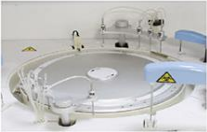
Reaction Tray: 37\pm 0.1^{\circ}\text{C} , water bath
