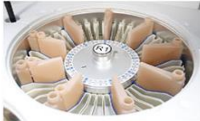
Reagent Tray: 2\sim 8^{\circ}\text{C} cooling for 24 hours
