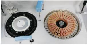
Mixer Probe Teflon coating to avoid cross contamination.
