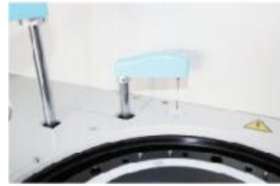
Mixer Probe Teflon coating to avoid cross contamination
