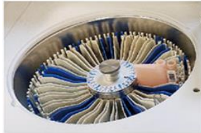
Reagent tray 2~8°C cooling for 24 hours
