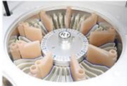
Reagent tray 2°C~8°C cooling for 24 hours
