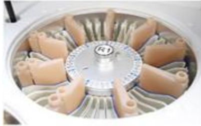
Reagent tray 2°C~8°C cooling for 24 hours
