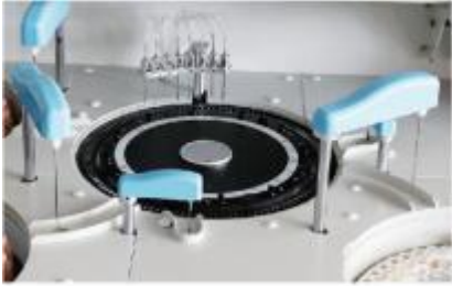
Reaction tray 37°C±0.1°C, real-time monitor
