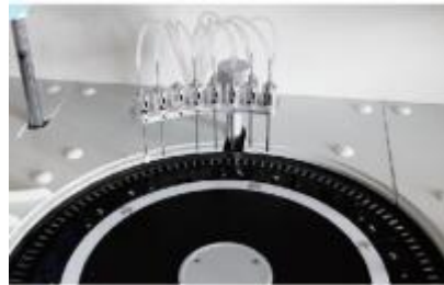
Washing Probe Independent 7-step washing system
