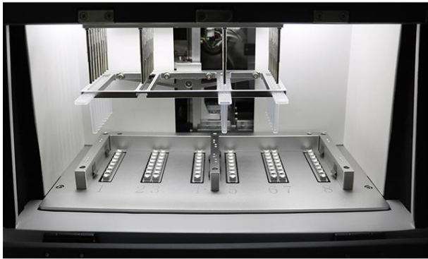
Concave design heating belt fits the deep hole tube Ensure rapid and uniform temperature rise
