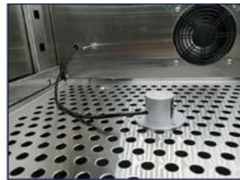
High water-proof grade Illumination Sensor
